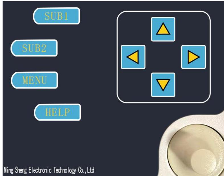
For the H2-1000KIII, use ↑ up, ↓ down, left or right ← to perform software operations. You can use up or down to select menu items. In addition, the instrument is equipped with an encoder, and all operations can be operated through the encoder. The encoder has three key states: left turn, right turn and Enter button (representing "confirm").
