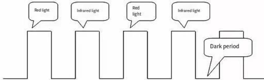
2. The timing sequence of red light and infrared light is fixed, as shown in the figure below: the luminous order of red light and infrared light can be interchanged, but the period is the same, the setting range is 200us-1ms, the dark period between red light and infrared light can be 200-1ms, and the luminous period between each group is fixed, which can be customized according to requirements, and the default can be set to 8ms.
