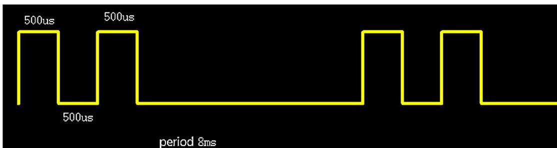
As shown in the figure above, the total period is 8ms, the red glow pulse is 500us, the infrared light emits after 500us interval, the period is also 500us, and then the rest of the cycle is all dark.
